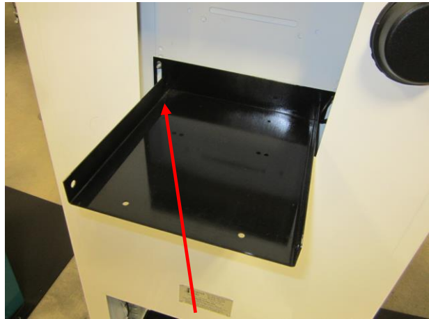
Bolt in the Top Slot for Mounting
