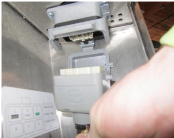
Disconnected Large Power Connector
