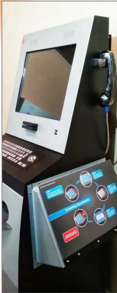
The Document Kiosk equipped with VoIP handset, credit card reader and scanner
