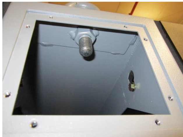
Opened Side Vent Showing Lifting Ring
